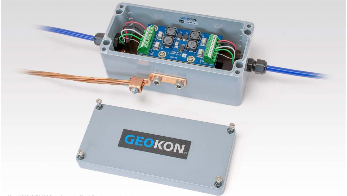
Model 4999-12LE LAB3 Surge Protection Circuit Board in protective enclosure.
